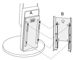
4. Pass the cables between (A) and (B), and align (B) with (A) to fit in.
