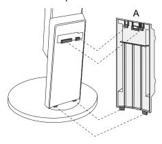
2. Slide (A) downward to secure the tabs to the attachment parts of the stand.
